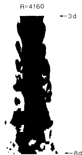
Fig. 10 Regions where the instantaneous concentration is greater than or equal to 40% of the maximum nozzle fluid concentration are shaded. The boundaries of these regions are contours where the concentration of the nozzle fluid is 0.40C_{\max} at R = 4160 .
